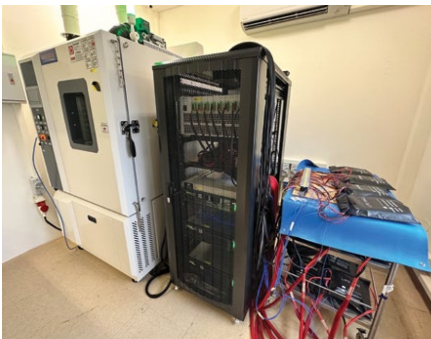
Battery testing chamber to perform degradation study for battery ageing, as part of the digital twin project.
